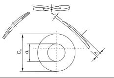
Applications : 1. Fasteners 2. Absorbing Vibrations 3. Compensation for Temperature Changes 4. Eliminating Side and End Play 5. Controlling End Pressure.
